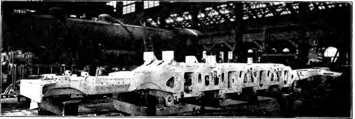
Side View of One-Piece Cast Steel Locomotive Bed for Southern Pacific Mountain Type Locomotive
